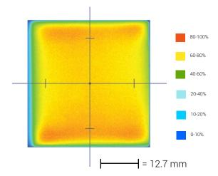
Optical measurement taken using BT050050-WHII3
