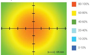
Optical measurement taken using FD0808-WHIIC @ 200mm
