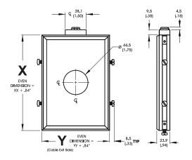
YY = WIDTH IN 1" EVEN INCREMENTS FROM 4" to 34" XX = HEIGHT IN 1" ODD INCREMENTS FROM 4" to 22"
