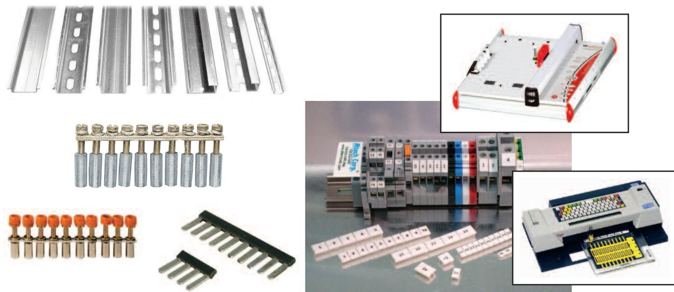
Last, but not least, the indispensable extras. End Stops prevent terminal blocks and other components from sliding laterally on the rail. End Plates close off the last terminal in a row of terminals. Isolation Partitions provide visual separation of terminal groups and ensure electrical isolation between adjacent terminals of different potentials. A wide selection of insulated and uninsulated ferules is offered for your applications and whenever stranded flexible wires must be terminated.
