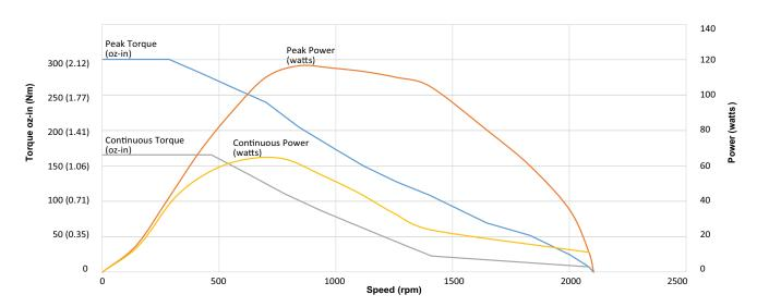
Continuous rating based on 25°C ambient temperature, motor mounted to a 6x6x¼ inch aluminum heat sink, and electronics/windings below maximum temperature. Peak torque is available for 3 seconds at a 10% duty cycle.
