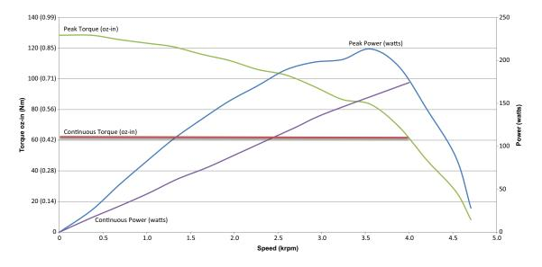
Continuous rating based on 25°C ambient temperature, motor mounted to a 6x6x¼ inch aluminum heat sink, and electronics/windings below maximum temperature. Peak torque is available for 3 seconds at a 10% duty cycle.
