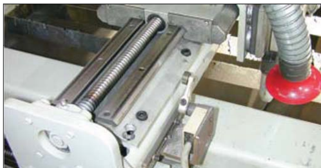
This "X-Y" Plasma cutter, using a LoPro ball screw driven system, operates in a harsh environment consisting of smoke, abrasive dust, weld splatter, hot sparks and elevated temperatures.
