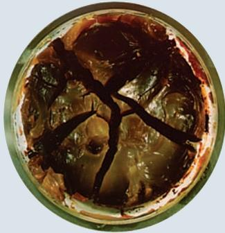
In an oven at 232 °C (448 °F) for 40 hours, the hydrocarbon lubricant had 40% weight loss.
