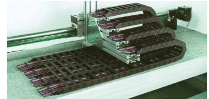
Example at igus® experimental laboratory: constant development and testing of Chainflex® electrical round cables
