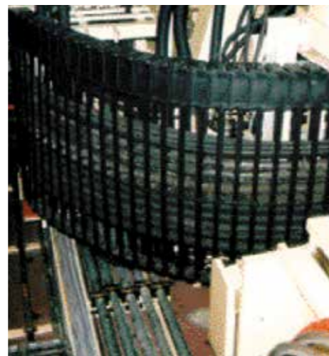
Hydraulics and electric cables are separated from one another in this example
