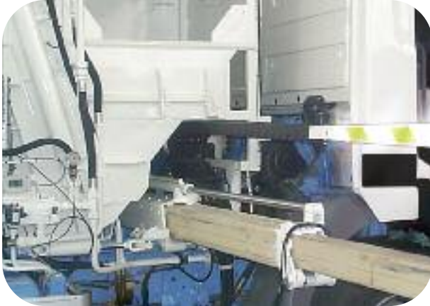
igus® ReadyChain® used for GEORG disposal vehicle - tested quality under tough conditions
