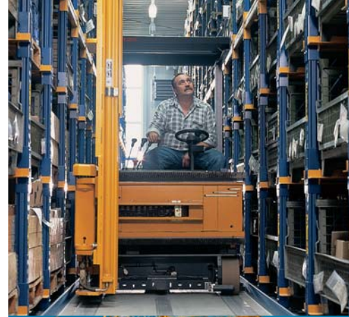
INDUSTRIAL TRUCKS ARE FITTED WITH SPRING-APPLIED BRAKES ON THE TRAVEL MOTOR AND WITH ELECTROMAGNETIC LOAD WHEEL BRAKES.
