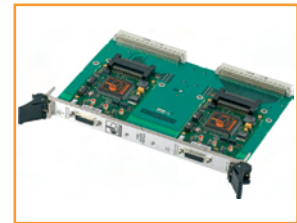
Dual axis VME configuration
