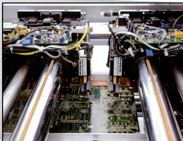
Automated circuit board tester - Probetest
