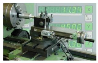
Fast and reliable linear feedback can be easily added to machines with the fitment of the LM10 linear magnetic encoder and a digital readout.
