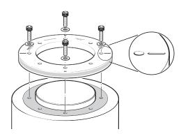
REXA rings are made with 4 fiducial points engraved onto the top surface, which simplify alignment.
