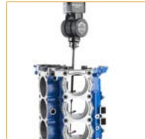
REVO™ – servo scanning head probing system
