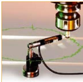
QC10 ballbar – fast machine tool performance testing
