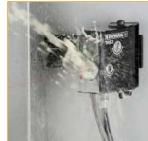
TRS2 – broken tool detection system
