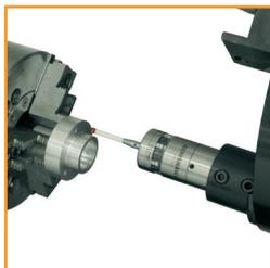
**Workpiece inspection probes** for automated measurement of component position and alignment.
