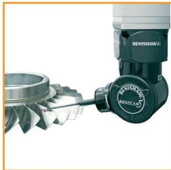
**REVO®** 5-axis high-speed scanning and multi-sensor inspection system.
